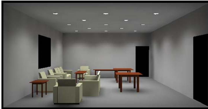
Existing Luminaires – No Day Lighting
